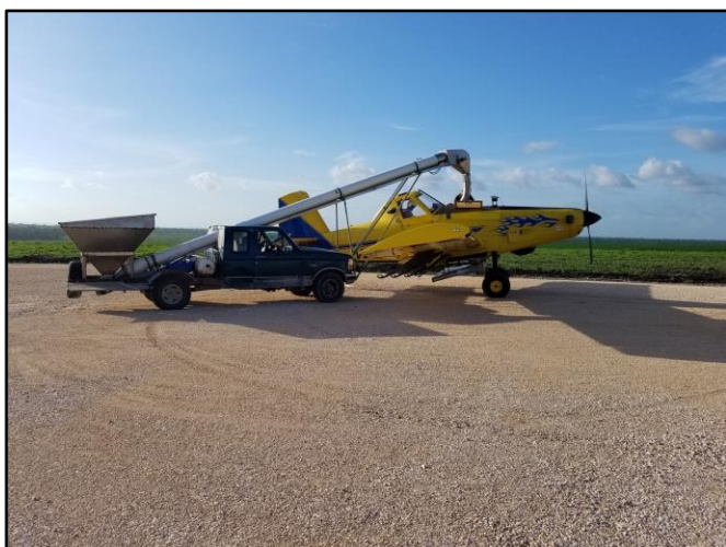
Fertilizer Aerial Application: Loading Air Tractor – Aug 10, '17 Time is of the essence: each minute costs $15.00!
