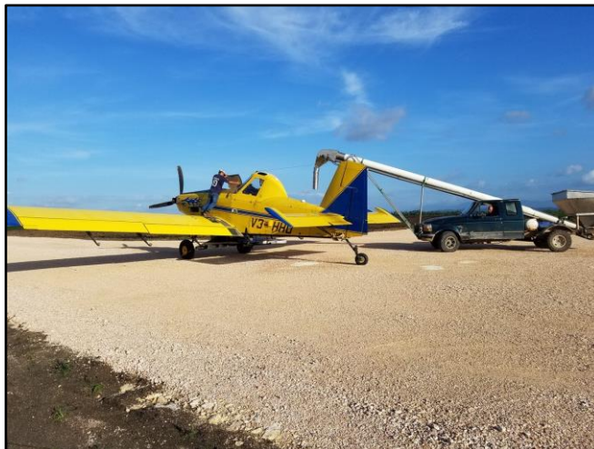
Fertilizer Aerial Application: Air Tractor ready! – Aug 10, '17 Each cycle fertilizes about 12 Ha (30 Acres) in 7.5 minutes
