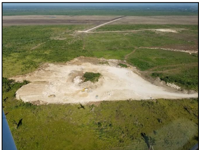
Local Source of Base Material – Feb 24, 2017 High Quality Gypsum provides base for roads/facilities
