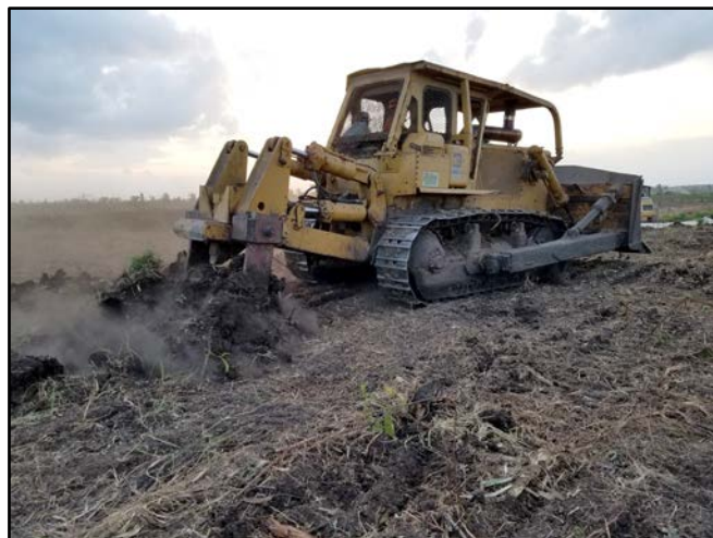
Subsoiling Trials – Apr 13, 2017 Blade is pulled 2 to 3 feet underground: every HP is needed!
