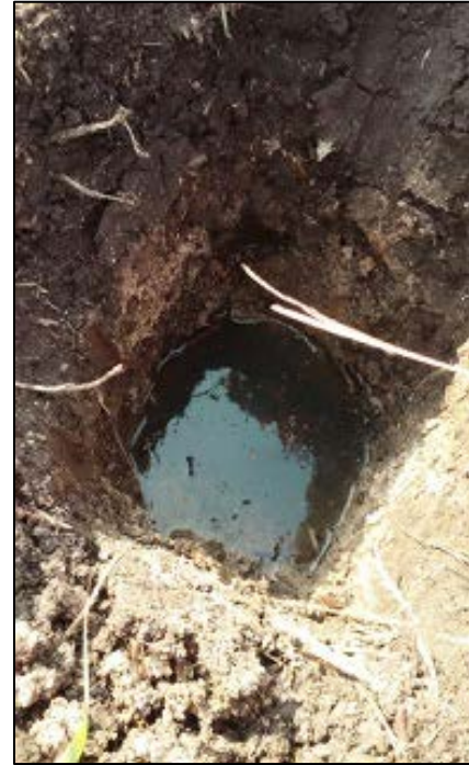
24 hours later Non-Subsoiled hole has 5.5 inches of water!
