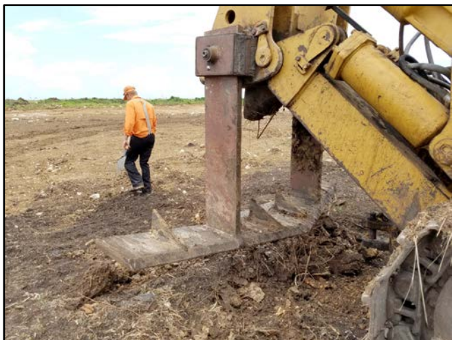
Subsoiling blade being trialed – Apr 13, 2017 Custom made blade is pulled by 500Hp D-9 bulldozer
