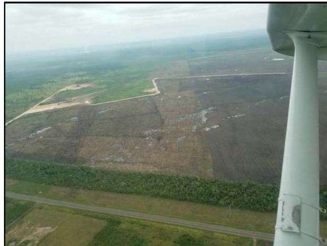
One week later after 100+mm of rain - Apr 24, 2017 Note the darker strip on left which was subsoiled: No ponding!
